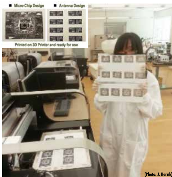
A student demonstrates silver conductors printed on 3D Printers in the Redfield Campus Renewable Energy Center.
